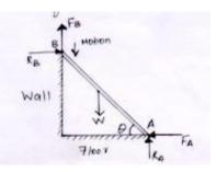
Let the angle of ladder with horizontal be  $\theta$  when the angle  $\theta$  exceeds angle of friction (or) when the weight of the man on the ladder makes instability to the ladder, the ladder slips down.
