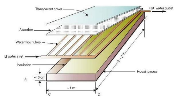
A collector is an independent unit which consists of: the absorber plate, the transparent cover and the insulation material bound together by a case that houses the collector components.
