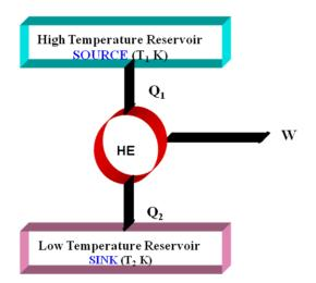
$Q_1$  = amount of heat supplied to steam in boiler from a high-temperature source.
