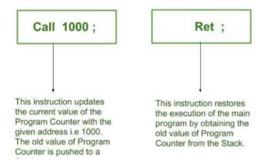
(3) It is important to note that the Main Program is suspended during the execution of any subprogram. Moreover, after the completion of the subprogram, the main program executes from the next sequential address present in the Program Counter.
