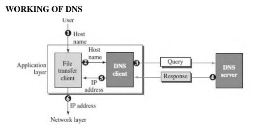
The following six steps shows the working of a DNS. It maps the host name to an IP address:
