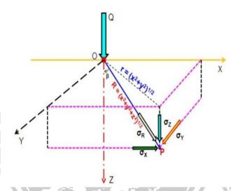
Let a point load act at a ground surface at a point O. which may be taken as a origin of x,y,z direction.
