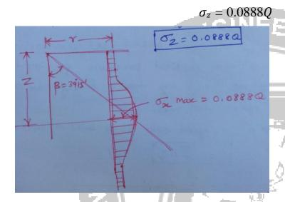
The vertical stress is <u>maximum</u> at the <u>centre</u> and <u>minimum</u> at the <u>corners</u>. The maximum stress is achieved at an angle of 39°15" of 0.0888Q
