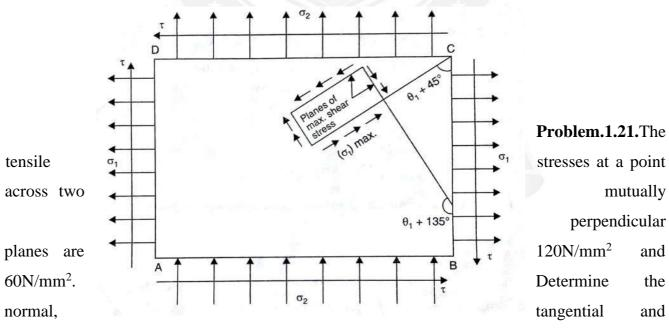
resultant stresses on a plane inclined at 30° to the axis of minor stress
