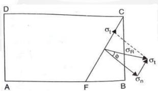
**Maximum Shear stress**. The shear stress is given by  $\sigma_t = \frac{(\sigma_1 - \sigma_2)}{2} \sin 2\theta$ . The shear stress
