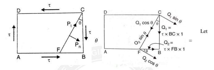
Angle made by oblique section FC with normal cross section BC,
