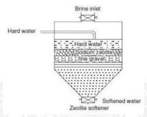
• Zeolite process results in *Zero hardness* – not suitable for public supplies – small amount is processed and mixed with unsoftened water to obtain standard limits.
