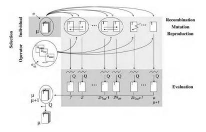
The above figure depicts the comma scheme where parents are not part of the selection pool. A notable extension of the GP evolution scheme is the operator pool, which contains a set of genetic operators, each attributed by a selection probability.
