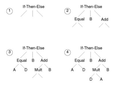
The above Figure illustrates the recursive, step-by-step construction of a random program term, an element of GPterm<sub>s</sub>- A symbol from S is randomly selected (If-Then-Else) as the root of the expression tree. At each of the branches, further subterms have to be composed by further random selection from S. This procedure is repeated until all leaf nodes are labeled with terminals.
