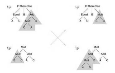
The above figure shows the simplest crossover version known as subtree exchange crossover, which is performed as follows: For each term a node is chosen at random. Inner nodes (including the root) as well as leaves are selectable. In Figure, the selected subtrees are marked by triangular shapes. The two recombined terms result from a mutual exchange of the selected sub-expressions.
