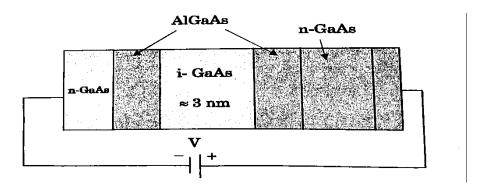
When electron energy is different from the energy of discrete state then the transmission is low. As E tends to  $E_n$  transmission will increase and becomes maximum when  $E=E_n$  After that as E increases the current will decrease. This decrease in current with increase in bias voltage is called negative resistance.
