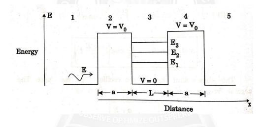
When the energy of incoming electron(E) is equal to one of the energy state of  $well(E_n)$ , the electron can tunnel through the barrier.
