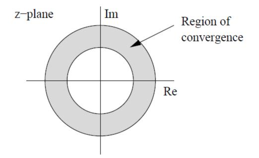
The inner radius of this ring may include the origin, and the outer radius may extend to infinity. If the ROC includes the unit circle |z| = 1, then the Fourier transform will converge.
