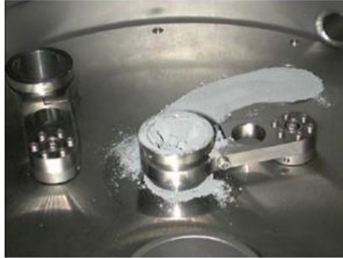
Fig 4.5 3D Micromac Powder Feed System. In this picture, only one of the powder feeders (located over the build cylinder) is filled with powder (courtesy: Laserinstitut Mittelsachsen e.V.
