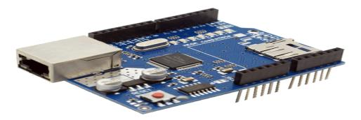
We can also connect another shield on the top of the Ethernet shield. It means that we can also mount two shields on the top of the Arduino board.
