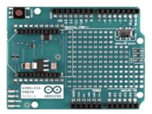
We can also solder the SMD (Surface Mount Device) ICs on the prototyping area. A maximum of 24 pins can be integrated onto the SMD area.
