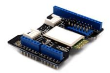
The communication distance of the Bluetooth shield is upto 10m at home without any obstacle in between.
