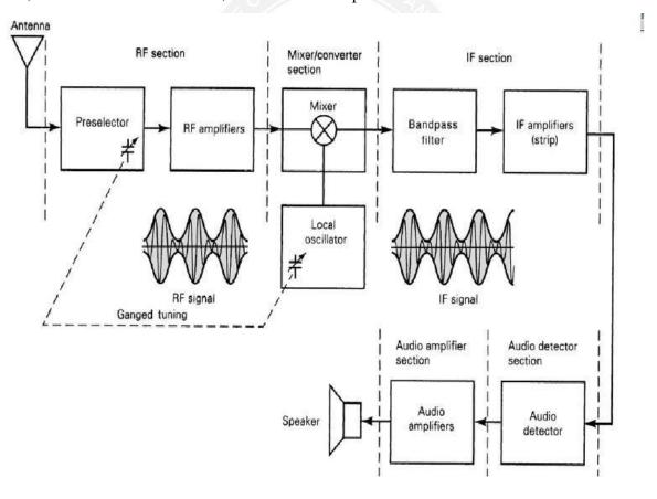
Fig 1.5.1 Superhetrodyne Receiver
