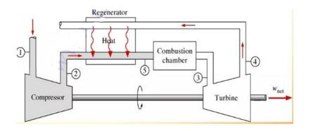
Temperature of the exhaust gas leaving the turbine is higher than the temperature of the air leaving the compressor.
