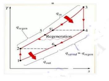
Regeneration process involves the installation of a heat exchanger in the gas turbine cycle. The heat- exchanger is also known as the recuperator. This heat exchanger is used to extract the heat from the exhaust gas. This exhaust gas is used to heat the compressed air.
