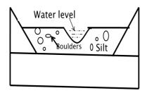
Deposits are made up boulders sand and silt of all grades
