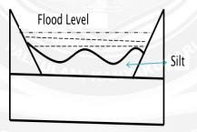
The flood deposit consist mostly of finest sand, silt and clay
