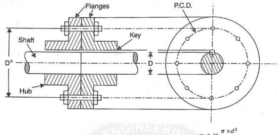
= Stress in bolt x Area of one bolt =  $q \times \frac{\pi \times d^2}{4}$
