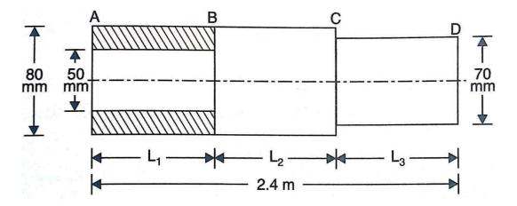
Let Shaft a AB = shaft 1, shaft BC = shaft 2 and shaft CD = shaft 3
