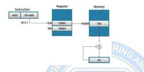
Here, we see that, in the Auto-decrement mode, the register R1 is decremented to 399 prior to execution of the instruction, means the operand is loaded to accumulator, is of address 1099H in memory, instead of 1088H.Thus, in this case effective address is 1099H and contents loaded into accumulator is 700.
