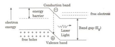
When the forward bias is increased, more and more photons are produced and it stimulates the recombination process in the release of photons in phase. The photons moving at the plane of the junction travels back and forth to grow its strength. After gaining enough strength, it gives out the laser beam of wavelength 8400 Å<sup>0</sup>.
