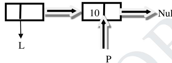
**Insert(20,L) -** A new node with data 20 is inserted and the next field is updated to NULL. The next field of previous node is updated to store the address of new node.
