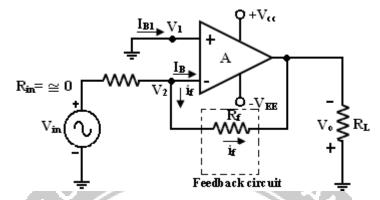
The input voltage drives the inverting terminal, and amplified as well as inverted output signal also applied to the inverting input via feedback resistor  $R_{\text{F}}$ .
