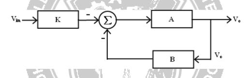
The comparison of eqn (15) with feedback (6) indicates that in addition to the phase inversion (sign), the closed loop gain of the inverting amplifier in K times the closed loop gain of the Non-inverting amplifier where K< 1. To derive a ideal closed loop gain, we can use Eqn 15 as follows, If AB >> 1, then (1+AB) = AB and  $A_F = K/B = -R_F/R_1 - ... - (16)$
