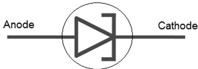
Fig:4.2.1 Symbol of Tunnel Diode
