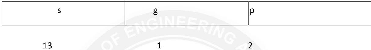
Where s designates the segment number, g indicates whether the segment is in the GDT or LDT, and p deals with protection. The offset is a 32-bit number specifying the location of the byte within the segment in question.
