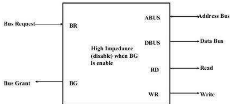
Fig 4: CPU bus signals for DMA transfer
