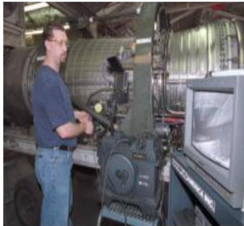
Fig: An inspector at Tinker Air Force base gets a magnified view of an engine's high-pressure turbine area with a new digital fiber-optic bore scope.
