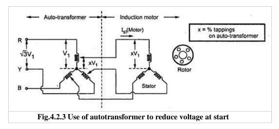
When motor gathers 80% of the normal speed, the change over switch is thrown into run position.
