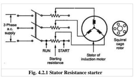
When the motor starts running, the resistances are gradually cut-off from the stator circuit. When the resistances are entirely removed from the stator circuit i.e. rheostats in RUN position then rated voltage gets applied to the stator. Motor runs with normal speed.
