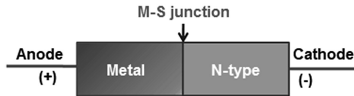
Fig:4.4.2 Metal-Semiconductor (M-S) Junction
