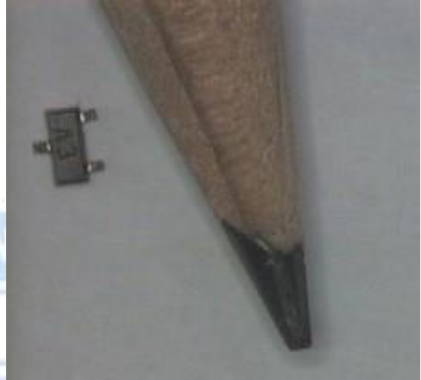
Figure 4: Equivalent circuit of a packaged Schottky diode and a photograph of a SOT23 packaged diode, with pencil tip for size reference
