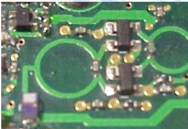
Figure 29: Photograph of a FET based switching mixer on and off in anti-phase with Q2 and Q4. The effect of this is that the RF signal and a 180° phase shifted version of the RF signal are alternately
