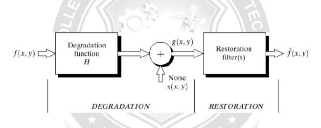
Fig3.1.1: A model of the image Degradation / Restoration process (Source: Rafael C. Gonzalez, Richard E. Woods, Digital Image Processing', Pearson, Third Edition, 2010.-Page-312)
