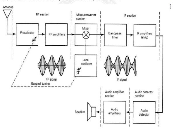
Fig 1.5.1 Superhetrodyne Receiver
