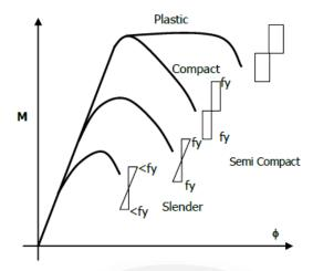
Class 2 (Compact): Cross – section, which can develop moment of resistance, but have inadequate plastic hinge rotation capacity for formation of plastic mechanism, due to lical buckling. The width to thickness rati of palte elements shall be less than that specified under class – 2 (compact), but greater than specified under class – 1 (Plastic)
