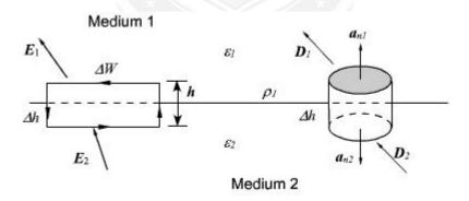
Fig 8.1: Boundary Conditions at the interface between two dielectrics (www.brainkart.com/subject/Electromagnetic-Theory\_206/)
