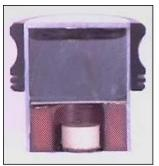
The <u>thickness of the active element</u> is determined by the desired frequency of the transducer. A thin wafer element <u>vibrates with a wavelength that is twice its thickness</u>. Therefore, piezoelectric crystals are cut to a thickness that is 1/2 the desired radiated wavelength. The higher the frequency of the transducer, the thinner the active element is.
