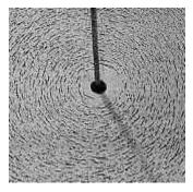
Also, the <u>direction of the magnetic field</u> is dependent on the <u>direction of the electrical</u> <u>current</u> in the wire. The direction of the magnetic field around a conductor can be determined using a simple rule called the "<u>right-hand clasp rule</u>". If a person grasps a conductor in one's right hand with the <u>thumb pointing in the direction of the current</u>, the <u>fingers</u> will circle the conductor in the <u>direction of the magnetic field</u>.
