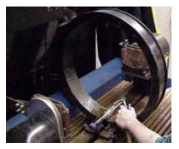
demagnetization feature is built in, which uses the coil and decaying AC.
