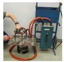
However, <u>caution is required</u> when using prods because electrical <u>arcing can occur</u> and cause <u>damage to the component</u> if proper contact is not maintained between the prods and the component surface. For this reason, the use of prods is not allowed when inspecting aerospace and other critical components. To help prevent arcing, the
