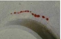
The advantage that a liquid penetrant inspection offers over an unaided visual inspection is that it <u>makes defects easier to see</u> for the inspector where that is done in two ways:
