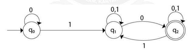
**Solution:** For the given transition diagram we will first construct the transition table.
