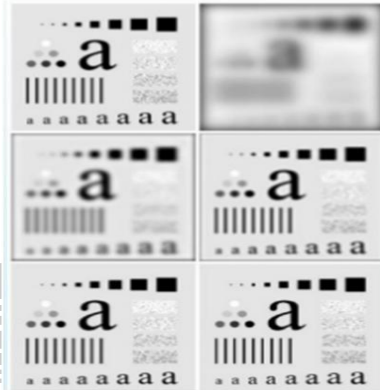
Fig. 2.2.3(a) Original image.(b)-(f) Results of filtering using BLPFs of order 2, with cutoff frequencies at the radii
