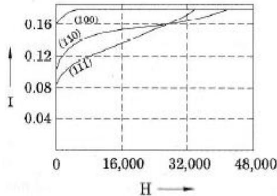
**Fig 3.6.3. Direction of magnetization**
