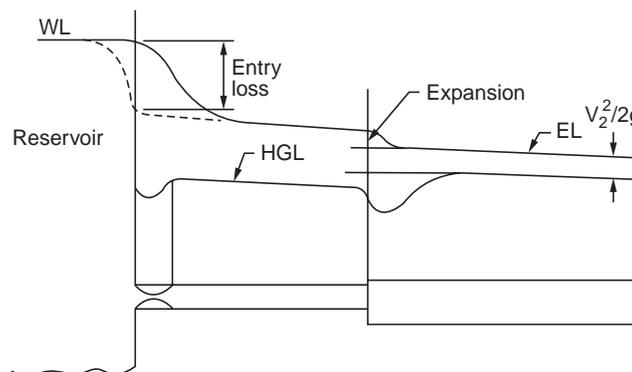
Figure 3.15.1 Energy and Hydraulic grade lines
