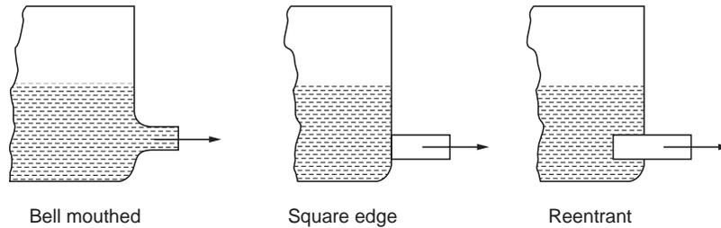
**(ii) Loss of head at submerged discharge:** When a pipe with submerged outlet discharges into a liquid which is still (not moving) whole of the dynamic head  $u^2/2g$  will be lost. The loss coefficient is 1.0. The discharge from reaction turbines into the tail race water is an example. The loss is reduced by providing a diverging pipe to reduce the exit velocity.
