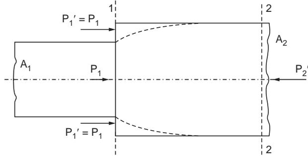
Applying conservation of momentum principle to the fluid between section 1 and 2, and denoting the actual pressure at section 2 as  $P_2'$ ,
