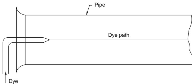
In turbulent flow there is considerable mixing between layers. A dye injected into the flow will quickly mix with the fluid. Most of the air and water flow in conduits will be turbulent. Turbulence leads to higher frictional losses leading to higher pressure drop. The friction factor is given by the following empirical relations.
