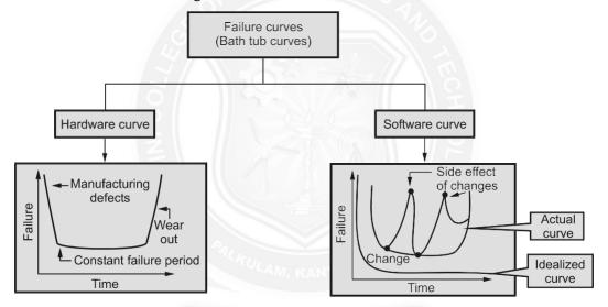
Failure curves for hardware and software
