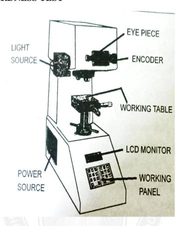
❖ The Vickers hardness test, used to determine quantitatively the indentation hardness of material under the application of a constant static load, is a widely accepted method for research work because it is capable of measuring hardness from very soft materials to extremely hard materials without changing the load or indenter.
