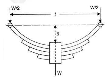
The above shows a laminated spring which consists of a number of parallel strip of a metal having different lengths and same width, placed one over the other. Initially all the plates are bent to the same radius and are free to slide one over the other. Fig. 16.11 shows the initial position of the spring, which is having some central deflection  $\delta$ . The spring rests on the axis of the vehicle and its top plate is pinned at the ends to the chassis of the vehicle.
