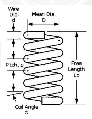
**Remove set:** The process of closing to a solid height a compression spring which has been coiled longer than the desired finished length, so as to increase the elastic limit.
