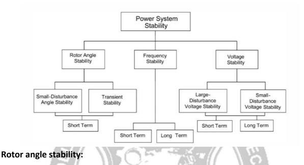
"It is the ability of the system to remain in synchronism when subjected to a disturbance". The rotor angle of a generator depends on the balance between the electromagnetic torque due to the generator electrical power output and mechanical torque due to the input mechanical power through a prime mover. Remaining in synchronism means that all the generators electromagnetic
