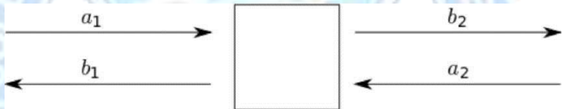
Figure 1.6 Signal Flow in a two port network
