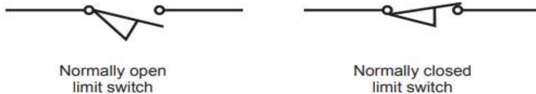
Fig. 4.13.4 Limit switches symbols
