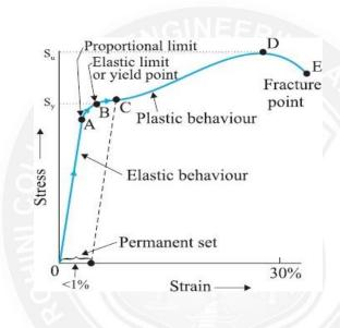
Fig.1.2.1 stress-strain diagram.
