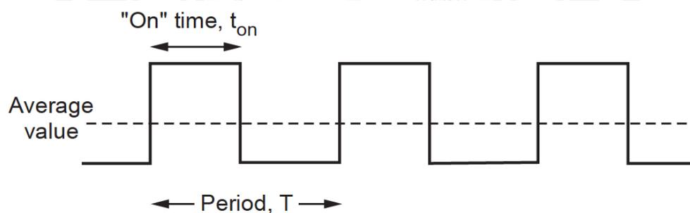
$$\text{Duty cycle} = 100 \% \times \text{Pulse on time} / \text{Pulse period}$$
