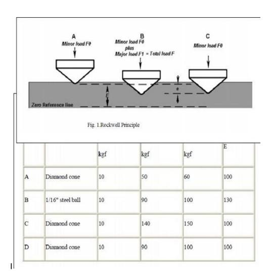
Fig 3.8.1(b) Indentation due to load
