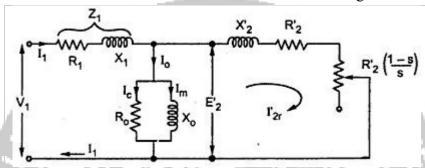
Fig. 3.28 Rotor equivalent circuit
