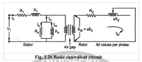
The stator and rotor sides are shown separated by an air gap.
