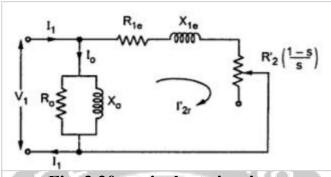
Fig. 3.30 equivalent circuit
