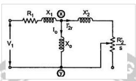
Fig. 3.31 Thevenin's Equivalent Circuit
