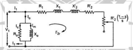
Fig. 3.29 Approximate equivalent circuit
