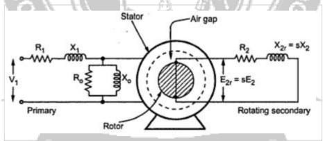
Fig. 3.25 Induction motor as a transformer
