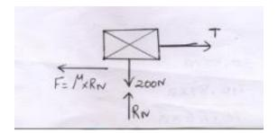
$\sum F_{Y}=0$   $R_{N} - 200 = 0$   $R_{N} = 200N$   $\sum F_{X} = m a$   $T = F = m \times a$   $T - \mu \times RN = \frac{200}{9.81} \times a$   $\mu = 0.3$  assume  $T - 0.3 \times 200 = 20.38 \times a$  $T - 60 = 20.38 \times a - ---->(1)$
