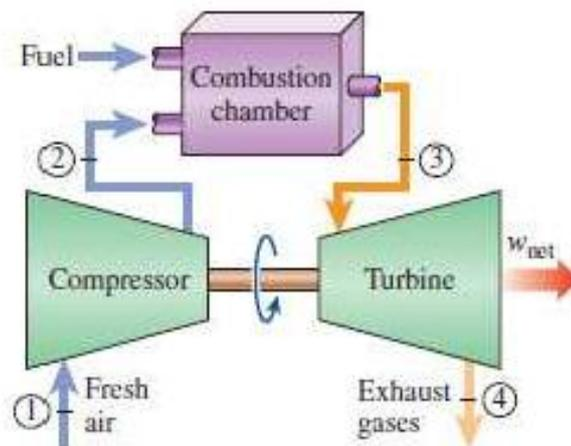
In the closed-gas turbine cycle, although the compression and expansion process have in common, combustion chamber is replaced by a heat exchanger in which increases the compressed air temperature. As given in Figure 2, ideal Brayton cycle is actually a closed-gas turbine cycle, and the steps of the Brayton cycle are like following;
