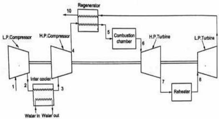
*Brayton cycle with intercooler, reheater and regenerator*
