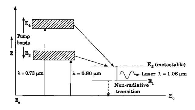
When the Krypton flash tube is switched on the  $Nd^{3+}$  ions  $\;$  present in the energy state  $E_0$  gains energy and moves to energy state  $E_4$  and  $E_3$
